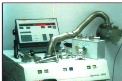
Helium MSLD Leak Detection System
