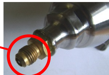
Connect a charge line to the schrader fitting - ensure the charge line includes a schrader valve depressor.
